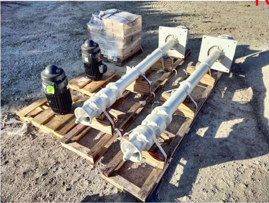
2024.08.02, Delivery of Vertical Turbine Pumps & Accessories
